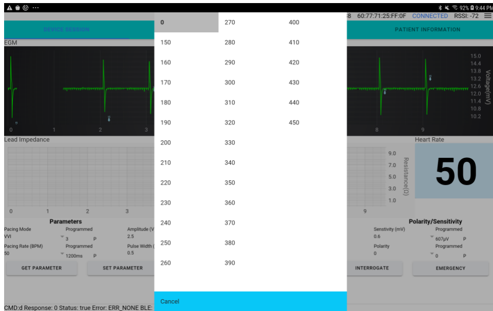
Figure 19: Blanking programmable range.
