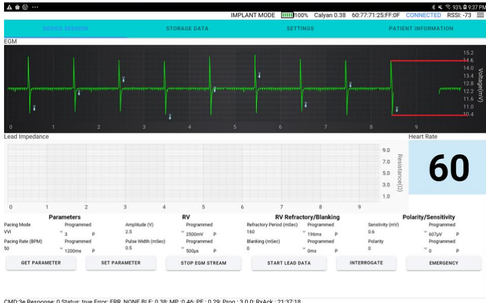
Figure 12 : R-Wave Amplitude Measurement
